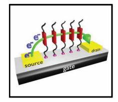
Highly reproducible n-type self-assembled monolayer field-effect transistors (SAMFETs) based on a perylene derivative are reported. Electron mobilities of  $1.5 \times 10^{-3} \text{ cm}^2 \text{ V}^{-1} \text{s}^{-1}$  and on/off current ratios up to  $10^5$  are obtained. By implementing n-type and p-type transistors in one device, a complimentary inverter based solely on SAMFETs is demonstrated for the first time.
